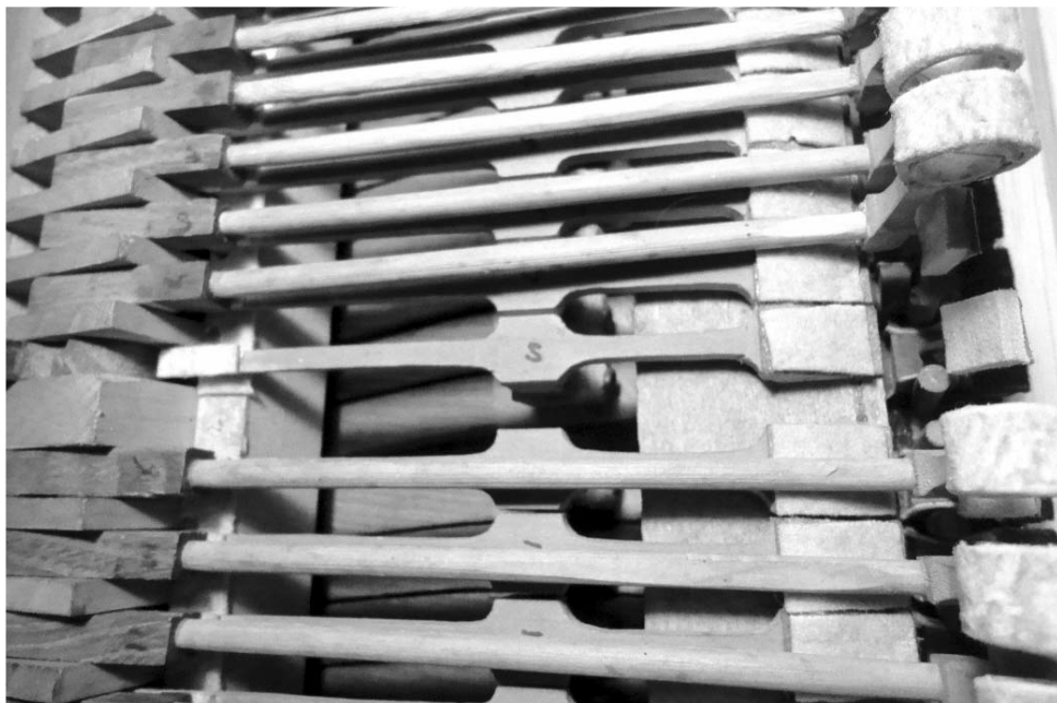
Figure 2. The intermediate levers from Ferrini's 1746 harpsichord-piano. Photo: Liuwe Tamminga.
